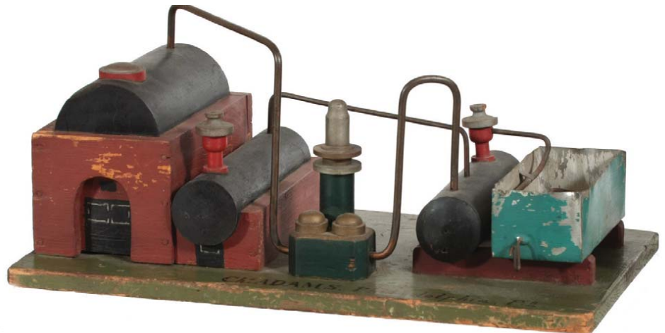
84).Patent Model. 6 x 13.25 x 7-3/8" Ca. 1866 painted wood and metal patent model for early oil refining station designed by Charles Adams, Philadelphia. Beautifully detailed, w/ nice early patina to paint surface and original 1865 tag on side. Has some scattered light wear, but overall attractive and displays very nicely (C. 8/-). Min. bid $100.
