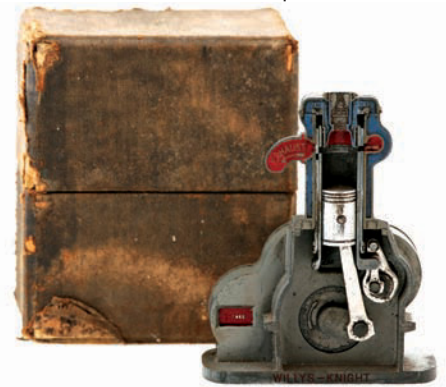
115).Willys-Knight Salesman's Sample. 4.25 x 3.25 x 1.75" early salesman's sample from Willys-Knight Automotive Co., featuring miniature version of metal engine compression chamber, w/ turning knob on backside that moves the piston up and down while at same time moving a descriptive red panel dial in bottom left display window. Very high quality piece, w/ fine detailing, as found still in its original presentation box (piece is excellent and all original, w/ tattering and fairly heavy wear to canvas/cloth material on outside of it's storage/presentation box). Min. bid $50.
