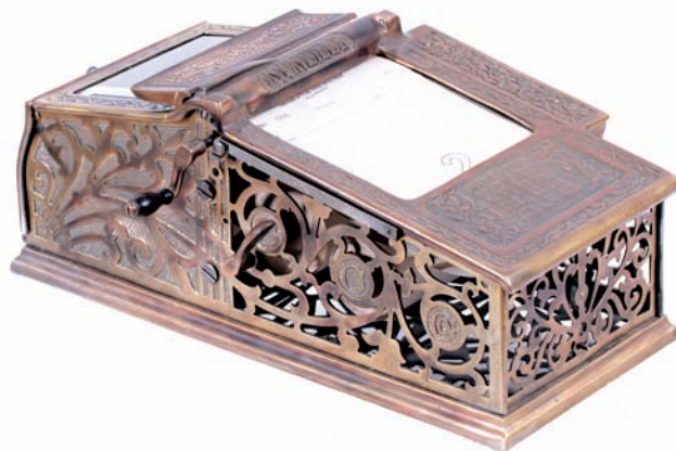
153). Receipt Registering Machine. 8 x 19 x 11" unusual, ca. 1890's Carter Crune Co. (Niagara Falls, NY) "Invincible" countertop mechanical receipt registering machine. Fancy, heavy, high quality all brass construction, w/ beautiful deep beveled viewing glass window at back. Has open space for writing on paper receipt, clerk would then crank handle and top 1/2 of receipt would come out of slot for customer and store copy would go into lock box while a new receipt automatically was loaded for next order. Excellent (see website addendum for further info). Min. bid $50.
