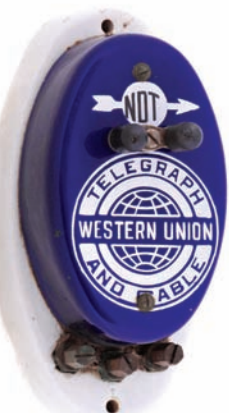
157). Western Union Call Box. 6-3/8 x 3-3/8 x 2.25" very early Western Union Telegraph and Cable Co. call box, w/ Co.'s early style logo. Heavy enameled porcelain covered piece is attached to white ceramic base w/ electrical mechanism inside and wind-up knob at top for notifying the local telegraph office to send over a messenger to retrieve a written message for sending as telegram. Excellent and all original (near mint), although wind-up mechanism is pretty temperamental. Min. bid $40.
