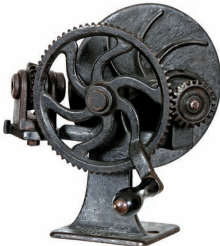
59) Gould & Cook Pencil Sharpener. 8.25 x 7 x 7.75" unusual, very early cast iron mechanical pencil sharpener (embossed Gould & Cook Co., Leominster, MA, w/ May 25 1886 patent date). Cranking handle moves three gear mechanism which rotates both pencil and the 5.75" (dia.) revolving iron disk holding sandpaper that shapes the pencil point. Excellent (nice working condition). Min. bid $50.
