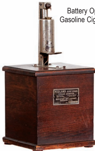
71). Midland Jump Spark Cigar Lighter. 15 (h) x 7 x 7" early Midland brand "Jump Spark" countertop cigar lighter (Davenport Mfg. Co., Davenport, IA). Has wooden mahogany base that hold 4 large dry cell batteries inside w/ original nameplate in front. Pushing down on nickel-plated metal lever creates a steady stream of electrical sparks which lights the wick of lighter providing open flame for cigar. Excellent overall and all original, w/ some light wear from use to metal plating (has original instructions on base). See our website addendum to find additional info and to view video of how piece works. Min. bid $100.
