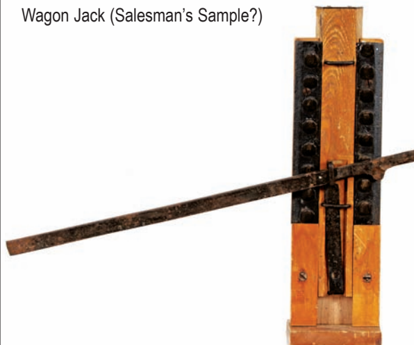
200).Salesman's Sample Wagon Jack. (18 x 5 x 5" wooden jack section- not including 23" long iron handle) important, very early, wood and cast iron working salesman's sample wagon jack from Buck & Co. (Lebanon, NH) w/ beautifully detailed stenciled advertising on backside. This is a substantial, heavy, very high quality piece that weighs almost 9 lbs. and appears to have been made for use as a salesman's sample, w/ a beautiful all original surface patina and a great country folk art look to it (mechanism works well). Excellent (C. 8+). Min. bid $100.
