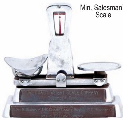
169).Miniature Salesman's Scale. 6 x 6 x 3" outstanding, early miniature candy scale, w/ advertising on both sides for "Exact Weight Scale Co." (Columbus, OH). This substantial, heavy, very high quality piece is an exact working miniature of one of Co.'s full size store scales and has a shiny chrome finish to its non-magnetic metal case- (bronze?) and weighs almost 6 pounds has engraving at bottom and was given as a presentation piece in 1951 to a Murphy Co. candy buyer. Neat piece!! Min. bid $50.
